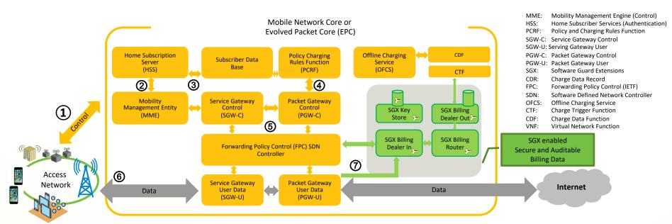
Fully secured and distributed Intel® Xeon based SGX protected CDR handling system Provides confidentiality and integrity of Charge Data Records (CDRs)
