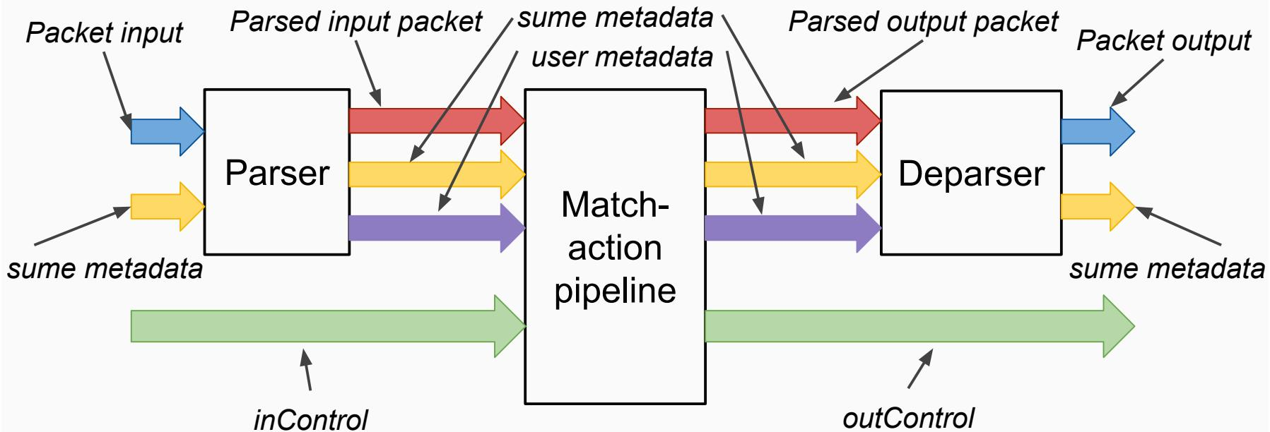
P4 used to describe parser, match-action pipeline, and deparser
