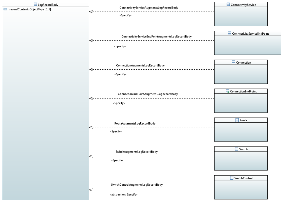
Figure 35 Example of Augmentation of the LogRecordBody with some classes from the model
